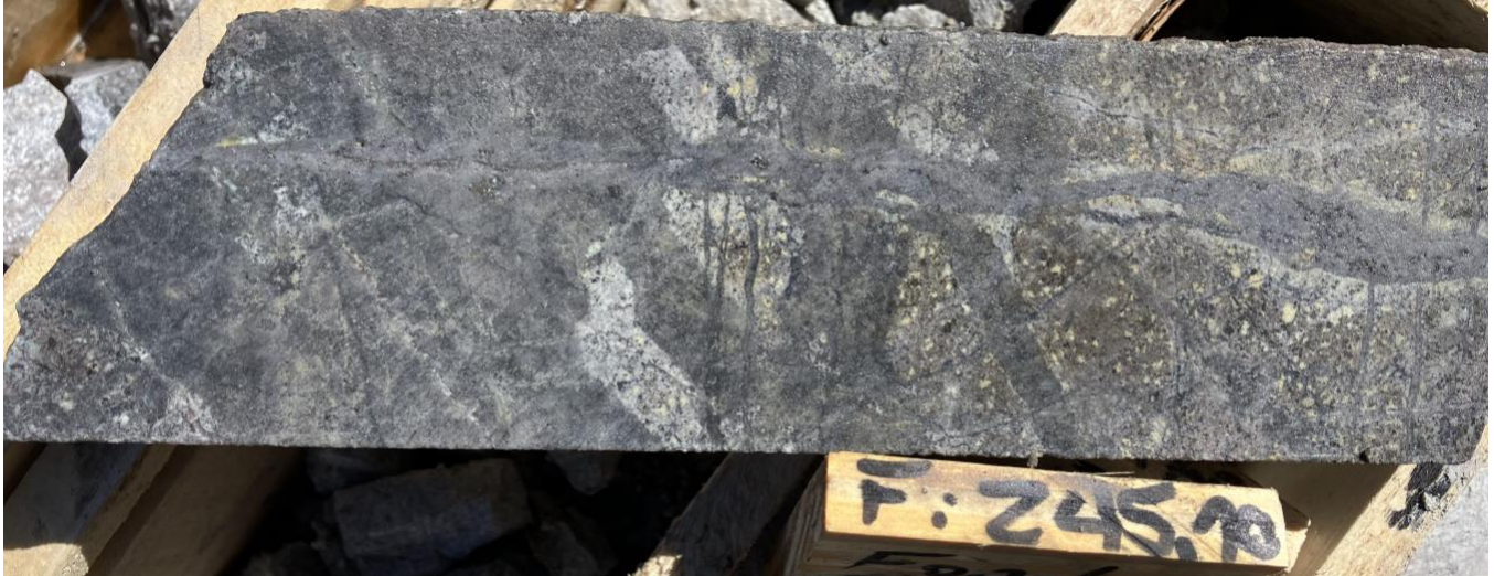
Image 2: Supergene Cu enrichment in porphyry A-type quartz stockwork veining with potassic (K-Spar) altered vein halos, overprinting early biotite altered quartz-diorite porphyry (245 m)
